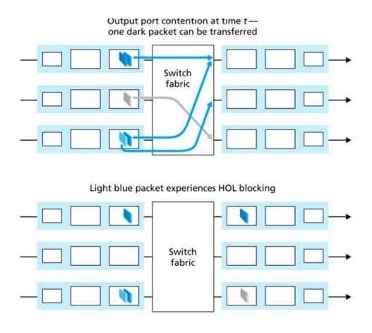
Second packet in bottom input port blocked, even though its output port is available, because first packet is blocked.
