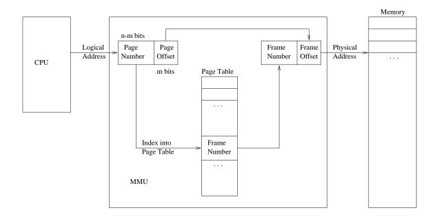
Virtual memory takes this one step further by removing the restriction that all logical addresses be mapped to physical addresses.
