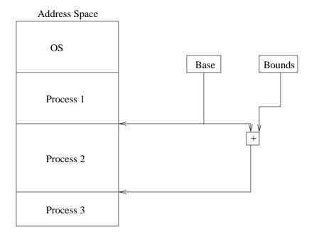
Multiple base/bounds pairs can be used to provide separate areas for the four memory segments associated with a program: code, heap, stack, and data.
