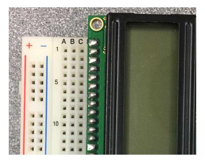
All of the pins in each of these bus columns are electrically connected, just like the pins in the numbered rows in the middle of the breadboard. Use these bus columns for the following power and ground connections to LCD display pins.
