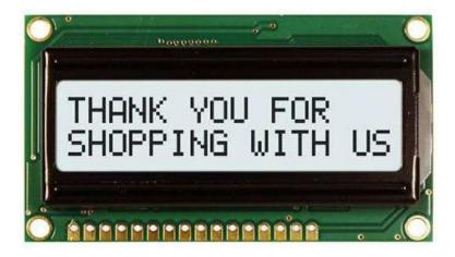
There are 16 connection pins along the bottom edge of the display's circuit board. Pin 1 is the leftmost pin and pin 16 is the rightmost pin. How do we know this? These two pin numbers are printed on the bottom of the circuit board:
