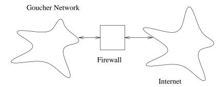
The Gibson Research web site is on the Internet. Thus, it would have tested the Goucher firewall and any firewall installed on the PC from which you ran their two tests. With the relationship diagrammed, the Gibson tests could indicate that you're safe when you might actually still be vulnerable. Why might you still be vulnerable?
