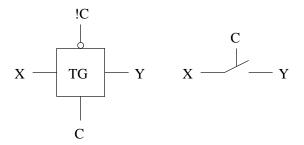
Typically used to enable writes onto a bus. For examples, two CPUs sharing a memory bus. Bus arbitration.
