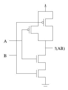
What determines power dissipation? Switching frequency.
