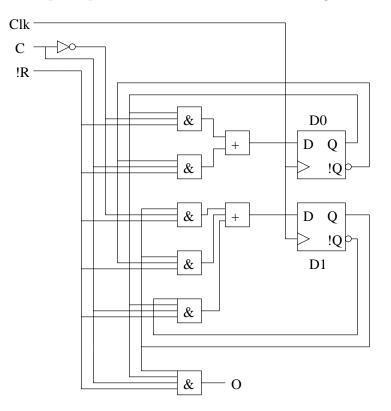
Determine input and output equations, state table, and state diagram for this circuit:
