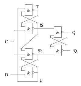
Analyze Q, !Q, !R, !S, T, and U with these input waveforms. Assume Q low initially.
