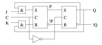
Analyze P, !P, Q, and !Q with these input waveforms. Assume Q low initially.
