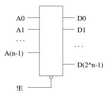
A circuit with n inputs. The inputs are interpreted as a binary number and used to select one of  $2^n$  output lines.
